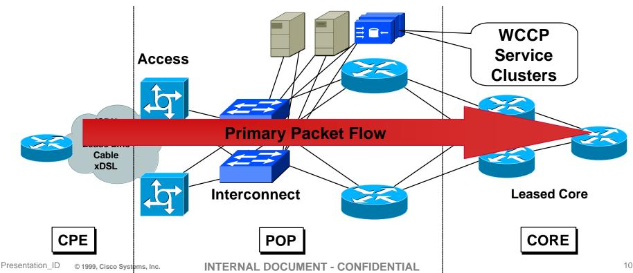
Work with the multi-level L2/L3 redundancy of the ISP POP. Equal paths in the IGP + **CEF leads packet asymmetry.**
