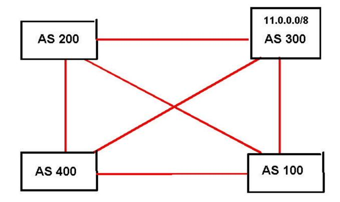
• Topology used to perform internal testing to study the effects when flapping the 11.0.0.0/8 prefix.
