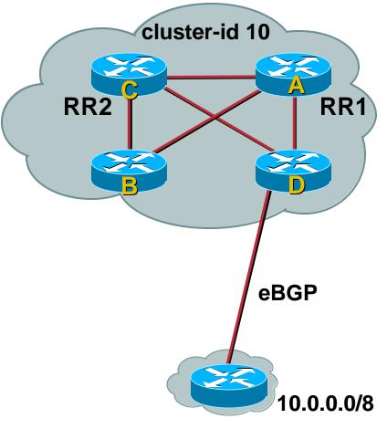
Lines Represent Both Physical Links and BGP Logical Connections
