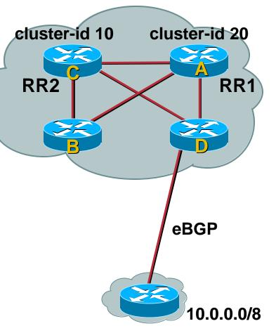
Lines Represent Both Physical Links and BGP Logical Connections
